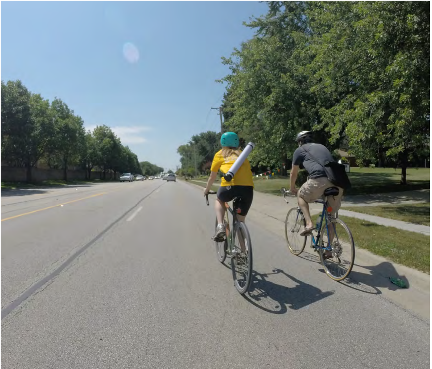
Wide, low traffic volume roadways, such as Westmore-Meyers Road, offer high potential to reallocate roadway width to other users.
