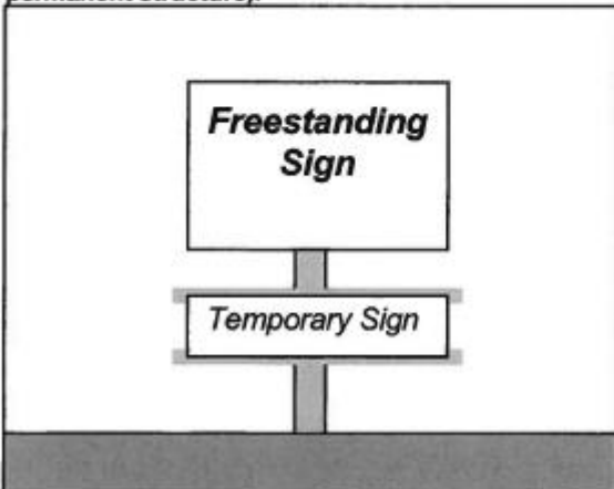
Figure 3. Permitted- Additional supports (which do not touch the ground) are used to affix a temporary sign at all corners to a freestanding sign (single permanent structure).
